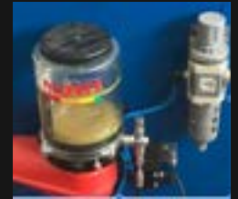
Electronically monitored central lubrication system
