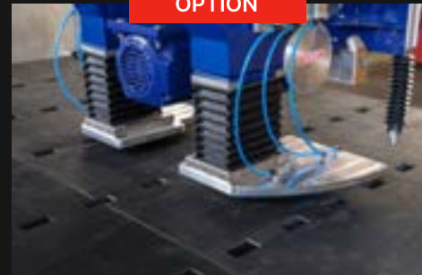
Vacuum Slab Lifter( 400kg cpt.) (software included )
